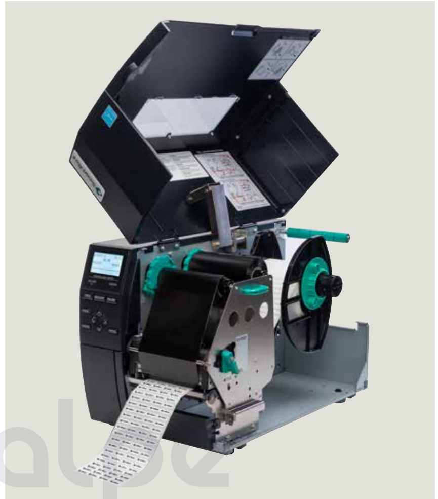
Internal detail with ribbon and consumables.
