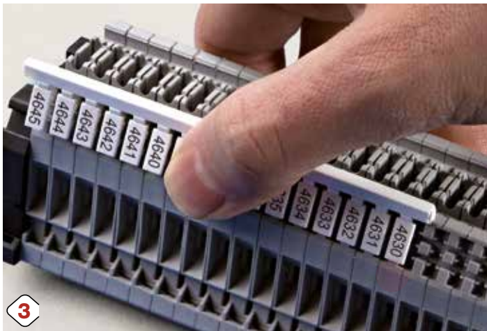
Insert the tags directly into the terminal block series using light pressure.
