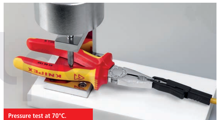
Testing the adhesion of the VDE insulating grips with 500 N at 70° C.
