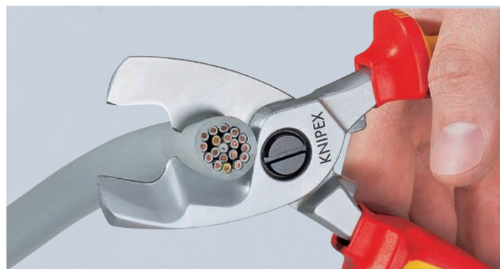
Final cut: after cutting the sheath in the front profile the conductors in the rear part are cut. Initial cut in the front profile, final cut in the rear profile - to keep it as easy as possible.
