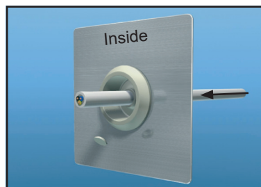
Pierce the grommet with the cable.
