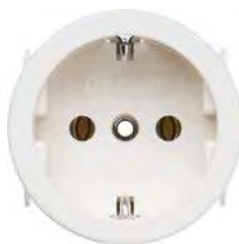
Built-in SCHUKO socket outlet with centre plate Ø 50 mm, SNAP IN 0.6 - 1.5 mm
