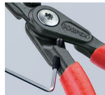
48 31 J1/J2 and 49 31 A1/A2: with overexpansion guard (adjustable using end stop), avoids overstretching of small internal circlips
